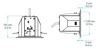
Once the Product is connected to a power source, push the side springs and insert in the opening made on the ceiling panel.
