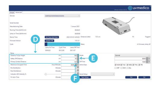
10) Save setup into template by pressing "Save Setup". A Name the template. This can be recalled whenever you have similar settings.
