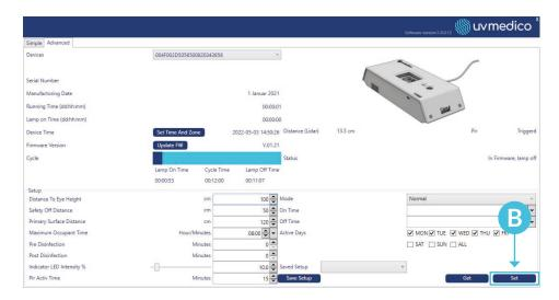
Once this information is saved and programmed into the unit, it is ready to test/start up.
